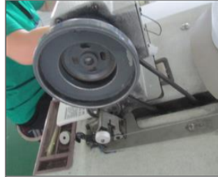
Photo of non-conformity The sewing machines in sewing section were not equipped with pulley guards.JPG
